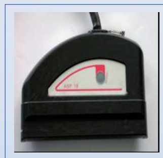
Figura 10. Transductor ASP 18. Pie medical. 3.5 MHz
